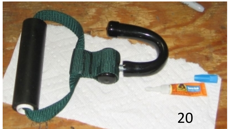
19. Insert a finished Hook Mount into the handle Hook Mount webbing and align the threaded hole with the hole in the webbing.
