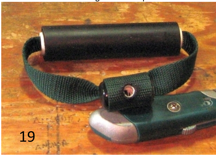
17. Punch a hole through the mark made in step #16. I use a 1/8" leather punch. I slip a 1" wood dowel through the Hook Mount webbing and set it up as shown.
